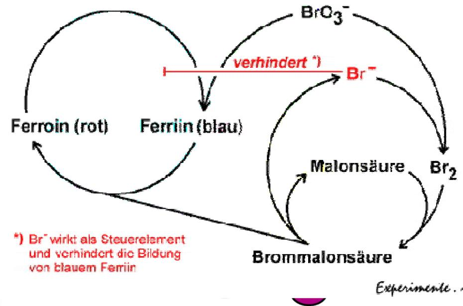
The reaction usually involves potassium bromate(VII) and malonic acid, optionally with cerium(IV) sulfate and citric acid. Ferroin is one of the common redox indicator
