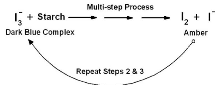
5. Eventually the faster step 3 becomes dominant and the change of  $\text{I}_3^-$  back to iodine/iodide stops after about 15 cycles, so the solution remains dark blue. The overall chemical reaction is:
