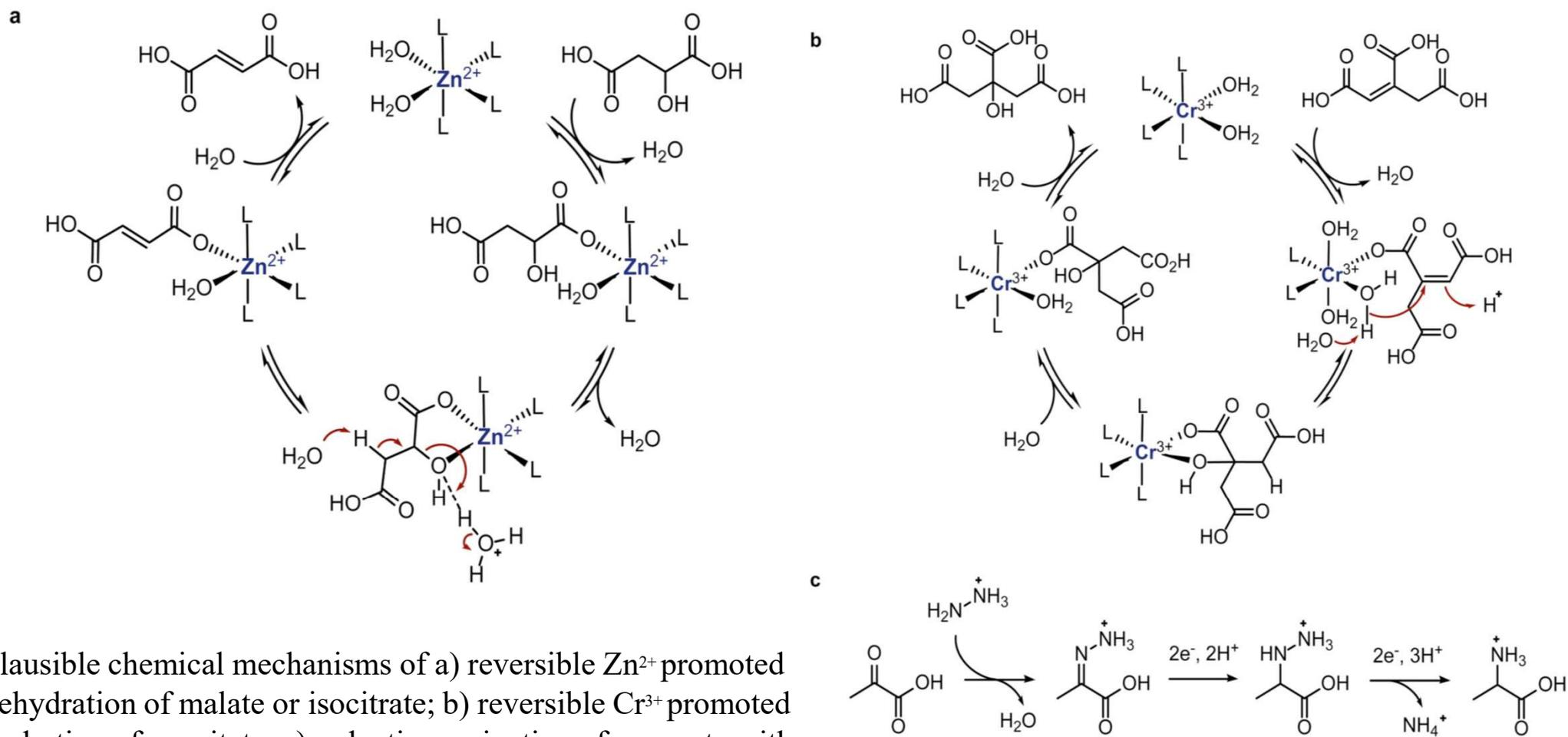
Plausible chemical mechanisms of a) reversible  $\text{Zn}^{2+}$  promoted dehydration of malate or isocitrate; b) reversible  $\text{Cr}^{3+}$  promoted hydration of aconitate; c) reductive amination of pyruvate with hydrazine and subsequent reductive N-N bond cleavage to generate alanine. Metal complexes are depicted as mononuclear species for clarity. L = undefined ligand
