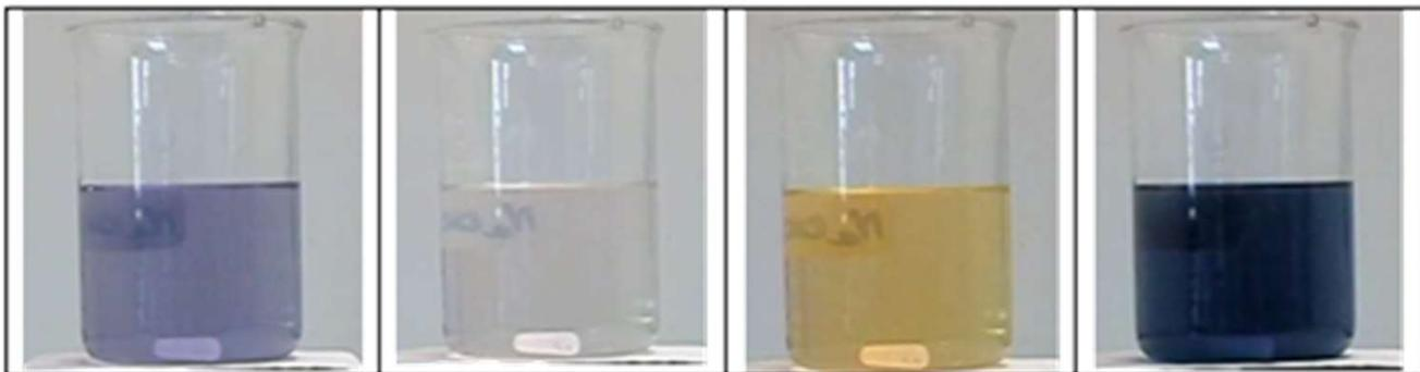
1. The iodate ion is changed into iodine by hydrogen peroxide. The color changes to amber:
