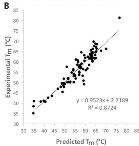
Plots of experimental versus predicted **(A)** free energy changes ( $\Delta G^{\circ}_{37}$ ) and **(B)** melting temperatures  $T_m$  for 94 SBZP-containing hachimoji DNA duplexes.
