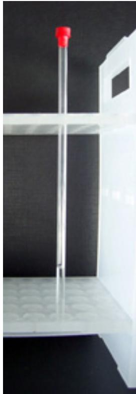
*After several minutes (to be sure wait for about one hour), when the gel is swollen enough and has reached the walls of the tube, you can put it into an upright position and let it stay so for several days for equilibration.*
