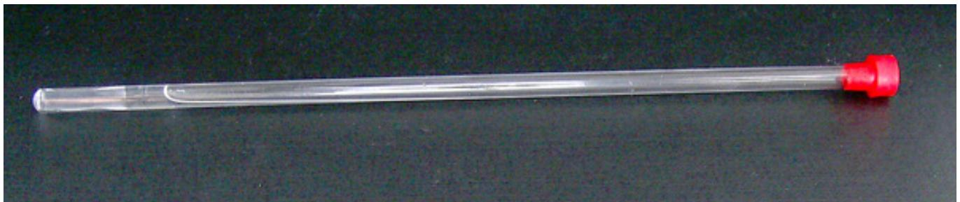
*...and then slowly put it into horizontal position, taking care, that the gel remains in the bottom part of the tube*
