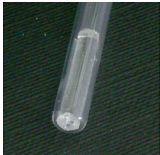
*Then simply push the polymer stick with a suitable long straw gently to the very bottom of the NMR tube.*
