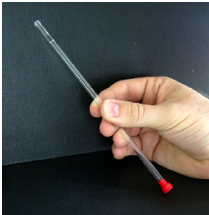
*If this nevertheless happened, act fast and simply turn the NMR-tube upside-down (make sure that the tube is sealed!) ...*
