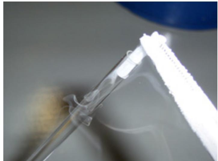
*To easily put the polymer stick inside the NMR tube, cool both the stick and the tube with liquid nitrogen or dry ice, then PDMS will not stick to the glass*
