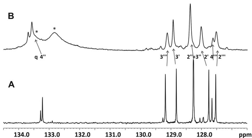
Figure 4. Gated decoupled  $^{13}\text{C}$  1D NMR spectra of the racemic mixture of compound **2** in isotropic  $\text{CDCl}_3$  solution (A) and in  $\text{PBLG}/\text{CDCl}_3$  (B). Assignment of the carbons according to the nomenclature defined in Figure 2 and corresponding chemical shift changes upon alignment are annotated. The difference in alignment tensors  $\mathbf{A}^R$  and  $\mathbf{A}^S$  apparently is not sufficient in this case to separate the two enantiomers.
