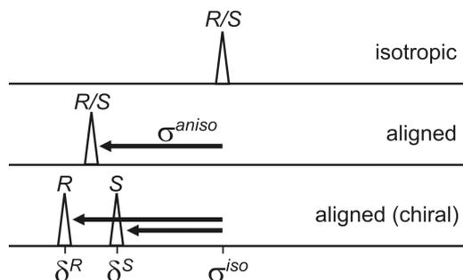
Figure 1. Schematic description of the effect of chiral alignment on chemical shifts. In the isotropic phase isotropic chemical shifts are observed that cannot distinguish enantiomers (top). When a sample is aligned in an achiral alignment medium, signals are shifted by RCSA, but *R* and *S* are still indistinguishable (middle). Alignment in a chiral alignment medium leads to two different RCSA values for the two enantiomers and eventually separates *R* from *S* (bottom).
